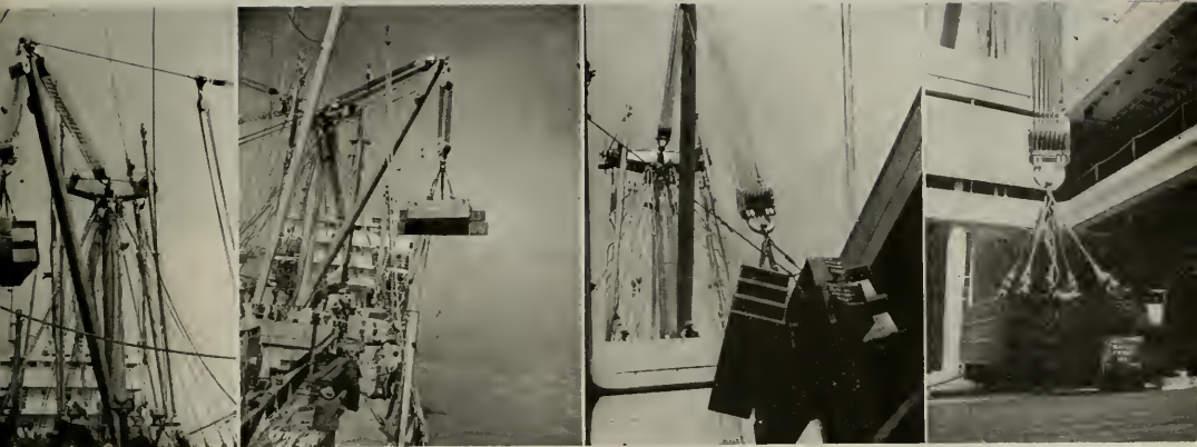
From left to right: A load of 71.5 long tons has been lifted from the wharf by ship's boom and is being hoisted inboard by forward offshore vang. Second from left: Test load outboard on port side. Vessel is listing at approximately 5°. Third from left: Test load on center line being lowered into hold. Last view: Test load at rest on bottom of hold.
